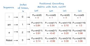
Positional Encoding Matrix for the sequence 'I am a robot'
